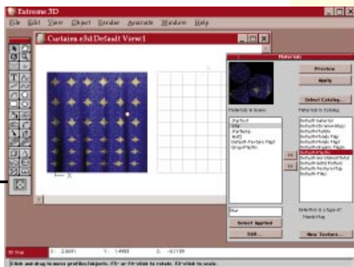
Fig 5 Extreme 3D, showing curtain with material applied. The grid next to it is the working plane used to draw profiles for 3D models
